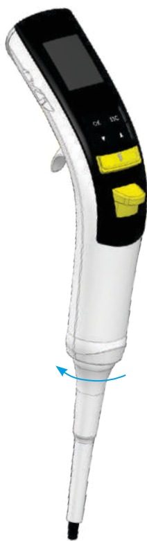
Step 1 Unscrew the Tip Ejector as per shown direction
